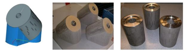
A joint cooperation with ENGIE Laborelec and CPC. Since 2017 the research center and technical service provider in electrical power technology and CPC have been working on the best process optimization to produce monolithic severe service Disk Stacks.
